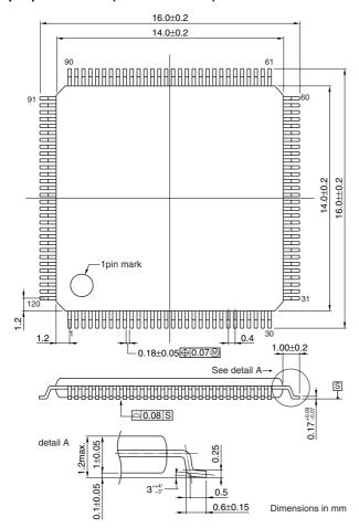
Each lead centerline is located within 0.07mm of its true position at maximum material condition.
