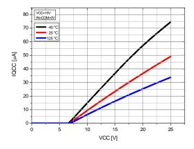
Figure 1. IQCC vs. Supply Voltage
