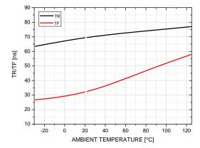
Figure 5. Rising/Falling Time vs. Temp.
