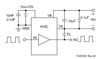
Figure 7. Switching Time Test Circuit
