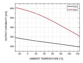
Figure 6. Output Sinking/Sourcing Current vs. Temp.
