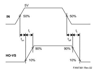
Figure 8. Input / Output Timing Diagram
