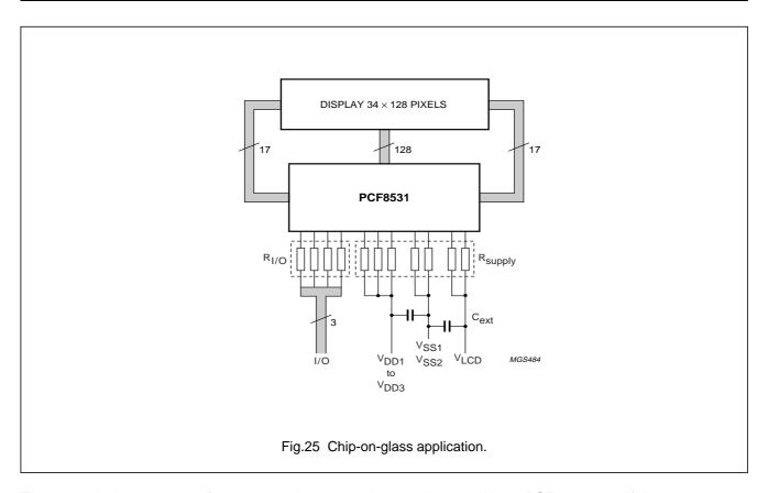
The required minimum values for the external capacitors in an application with the PCF8531 are as follows:
