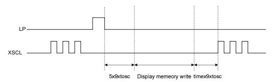
The allowable writing duration is since "5 x 9 x  $t_{OSC}$ " has elapsed ( $t_{OSC}$  = 1/ $f_{OSC}$ : a cycle of the oscillation frequency) from the positive going edge of LP up to {(TCR) – (C/R) – 7} x 9 x  $t_{OSC}$ .
