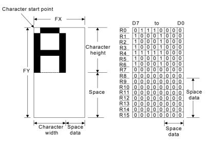
Figure 7-9: Example of Character Display ([FX]  $\leq$  8) and Generator Bitmap
