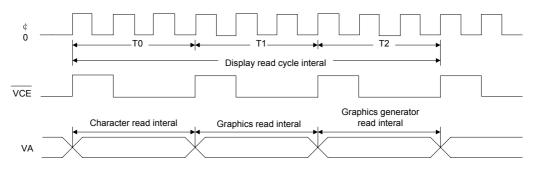
Figure 7-15: Display Memory Basic Read Cycle
