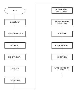
Figure 8-1: Initialization Procedure
