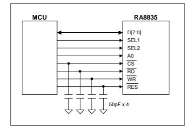
Figure A-1: Connection of MCU and RA8835
