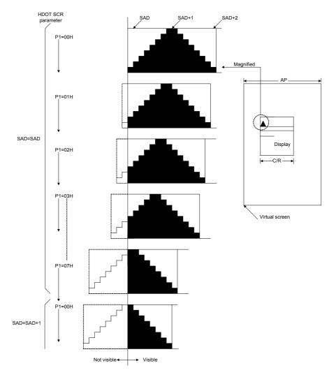
Note that the HDOT SCR command cannot be used to scroll individual layers.
