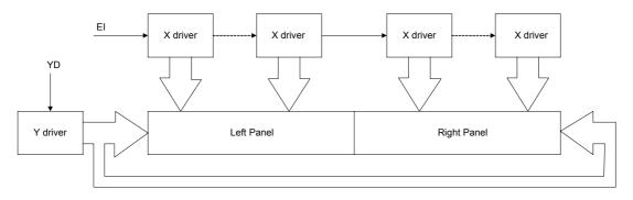
Figure 6-4: Left-and-Right Two-panel Display
