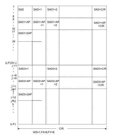
Figure 7-14: Two-panel Display Address Indexing
