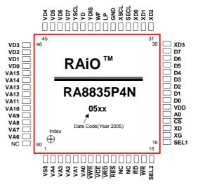
Figure 4-2: RA8835P4N (TQFP-60 Pin)
