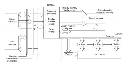
Figure 8-5: System Block Diagram
