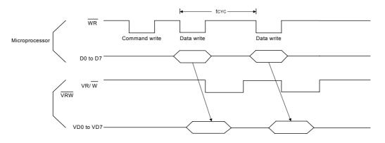
Figure 7-1A: Display Memory Write Cycle
