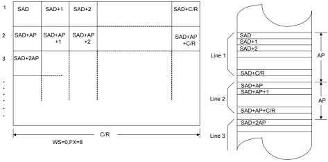
Figure 7-13: Character Parameters vs. Memory Note: One bit of display memory corresponds to one pixel.
