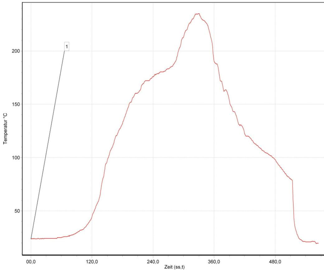
**Abbildung 1:** Example of a temperature curve – Attention, has to be adapted corresponding to the conditions on the motherboard.
