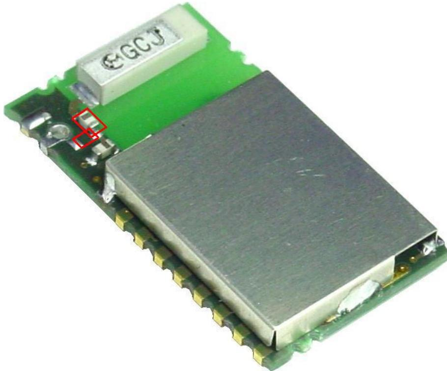
The AMB2300 can be operated also with an external antenna. In addition the red marked condenser (100pF 0603) must, as are changed above shown in its position. The lateral antenna connection is available then for a coaxial cable or a wire antenna.
