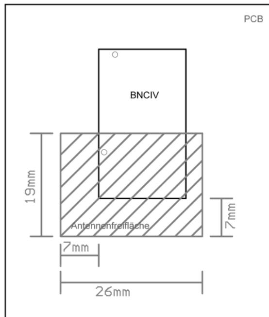
The BNC4 is not isolated, so even if there are normally no short circuit problems, because of the solder resist, an isolation should be placed between BNC4 and motherboard in case of any copper on the top side of the motherboard underneath the BNC4.
