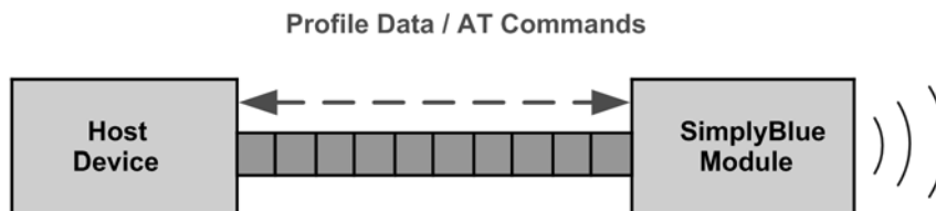
Profile Data Sent/Received To/From the SB module
