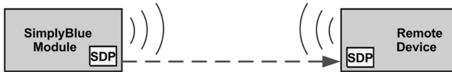
SB device initiates the SPP link establishment
