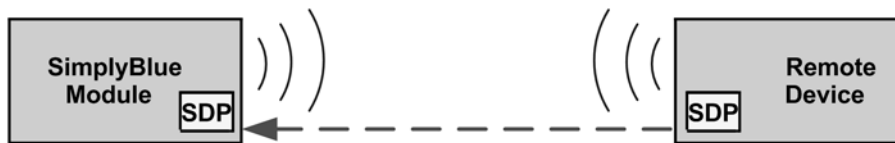
Remote device initiates the SPP link establishment
