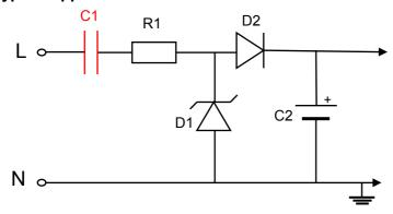
Example of connection in series with the main power supply (C1). Typical applications include energy meters, household appliances, etc.
