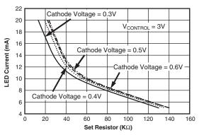
FAN5614 LED Current vs. Set Resistor
