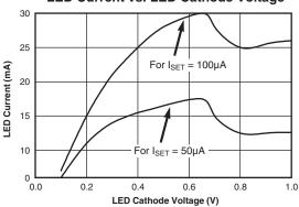
FAN5614 LED Current vs. LED Cathode Voltage
