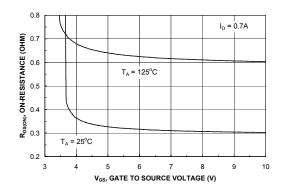
Figure 3. On-Resistance Variation with Temperature.
