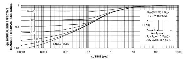
Figure 11. Transient Thermal Response Curve.
