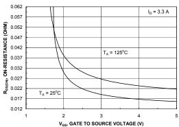
Figure 3. On-Resistance Variation with Temperature.
