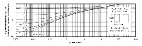
Figure 11. Transient Thermal Response Curve.
