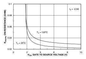
Figure 4. On-Resistance Variation with Gate-to-Source Voltage.
