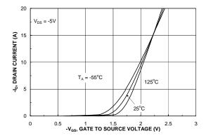
Figure 5. Transfer Characteristics.
