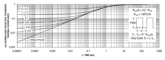
Figure 11. Transient Thermal Response Curve.
