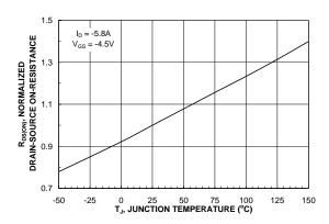
Figure 3. On-Resistance Variation with Temperature.
