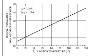
Figure 3. On-Resistance Variation with Temperature.
