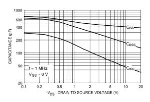
Figure 8. Capacitance Characteristics.
