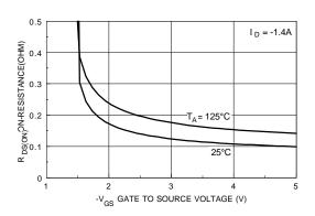
Figure 4. On-Resistance Variation with Gate-To-Source Voltage.
