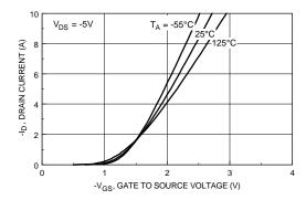
Figure 5. Transfer Characteristics.
