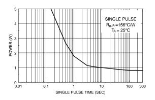
Figure 10. Single Pulse Maximum Power Dissipation.
