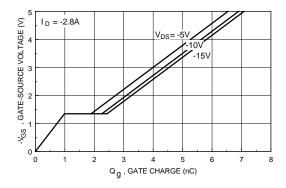
Figure 7. Gate Charge Characteristics.
