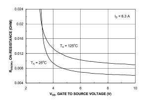
Figure 3. On-Resistance Variation with Temperature.
