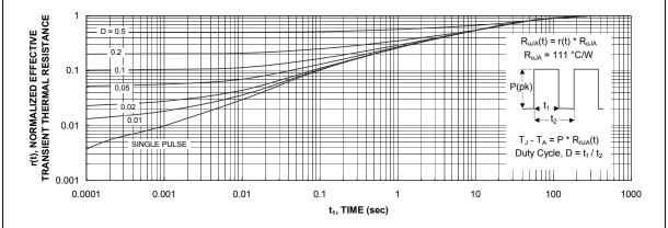
Figure 11. Transient Thermal Response Curve.
