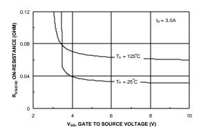
Figure 3. On-Resistance Variation with Temperature.
