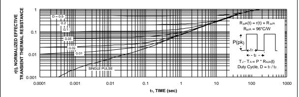
Figure 11. Transient Thermal Response Curve.
