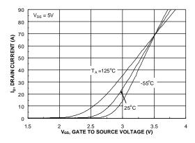
Figure 5. Transfer Characteristics
