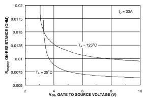
Figure 4. On-Resistance Variation with Gate-to-Source Voltage
