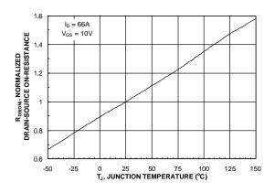
Figure 3. On-Resistance Variation withTemperature
