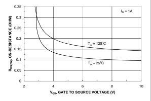
Figure 4. On-Resistance Variation with Gate-to-Source Voltage.
