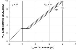
Figure 7. Gate-Charge Characteristics.
