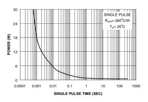
Figure 10. Single Pulse Maximum Power Dissipation.
