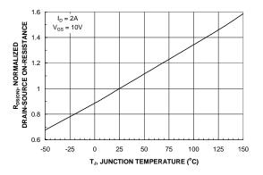
Figure 3. On-Resistance Variation with Temperature.
