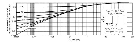
Figure 11. Transient Thermal Response Curve.
