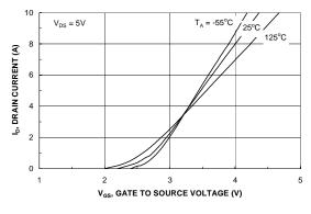
Figure 5. Transfer Characteristics.
