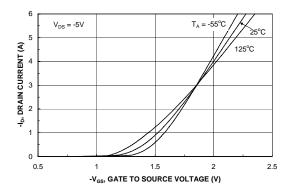
Figure 5. Transfer Characteristics.
