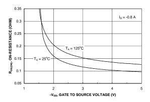
Figure 4. On-Resistance Variation with Gate-to-Source Voltage.
