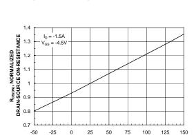
Figure 3. On-Resistance Variation with Temperature.
