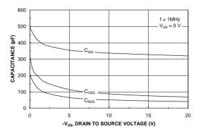
Figure 8. Capacitance Characteristics.
