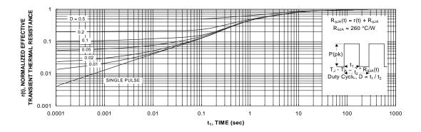
Figure 11. Transient Thermal Response Curve. Thermal characterization performed using the conditions described in Note 1c. Transient themal response will change depending on the circuit board design.
