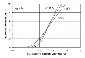
Figure 5. Transfer Characteristics.
