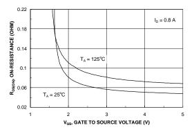
Figure 4. On-Resistance Variation with Gate-to-Source Voltage.
