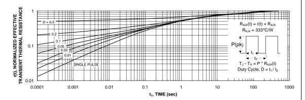
Figure 11. Transient Thermal Response Curve.
