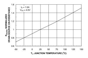
Figure 3. On-Resistance Variation with Temperature.
