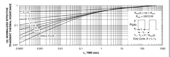
Figure 11. Transient Thermal Response Curve.
