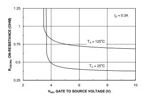
Figure 3. On-Resistance Variation with Temperature.
