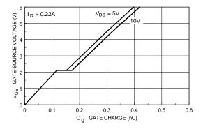
Figure 7. Gate Charge Characteristics.
