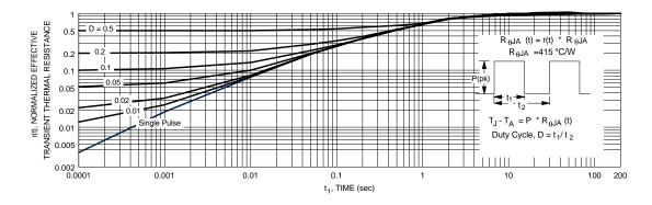
Figure 11. Transient Thermal Response Curve.
