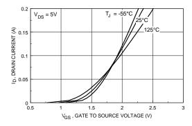
Figure 5. Transfer Characteristics.
