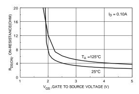
Figure 4. On-Resistance Variation with Gate-to-Source Voltage.
