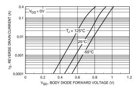
Figure 6. Body Diode Forward Voltage
