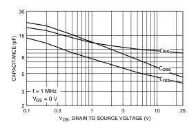
Figure 8. Capacitance Characteristics.
