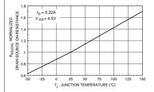
Figure 3. On-Resistance Variation with Temperature.
