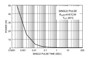
Figure 10. Single Pulse Maximum Power Dissipation.
