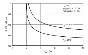
Figure 3. On-Resistance Variation with Input Voltage.
