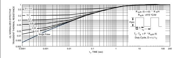
Figure 4. Transient Thermal Response Curve.
