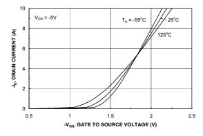
Figure 5. Transfer Characteristics.
