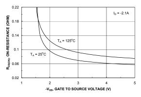
Figure 4. On-Resistance Variation with Gate-to-Source Voltage.
