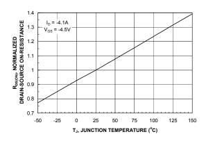
Figure 3. On-Resistance Variation withTemperature.
