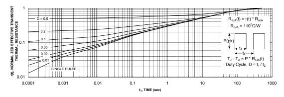
Figure 11. Transient Thermal Response Curve.
