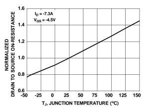
Figure 3. Normalized On-Resistance vs Junction Temperature
