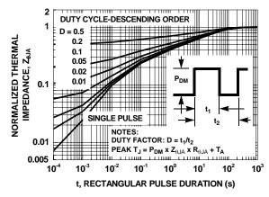
Figure 12. Transient Thermal Response Curve
