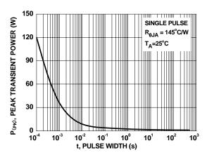
Figure 11. Single Pulse Maximum Power Dissipation
