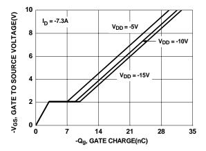
Figure 7. Gate Charge Characteristics
