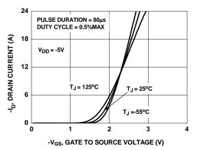
Figure 5. Transfer Characteristics
