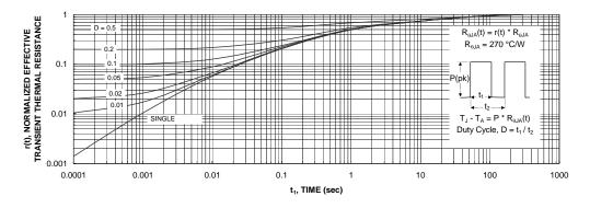
Figure 11. Transient Thermal Response Curve.
