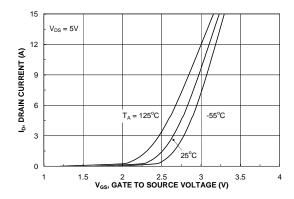
Figure 5. Transfer Characteristics.
