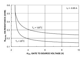
Figure 3. On-Resistance Variation withTemperature.
