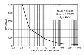
Figure 10. Single Pulse Maximum Power Dissipation.
