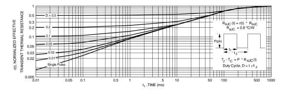
Figure 11. Transient Thermal Response Curve.
