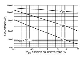
Figure 8. Capacitance Characteristics.
