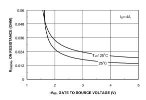
Figure 3. On-Resistance Variation with Temperature.
