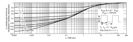
Figure 11. Transient Thermal Response Curve.
