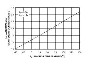
Figure 3. On-Resistance Variation with Temperature.
