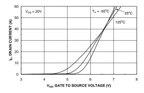
Figure 5. Transfer Characteristics.
