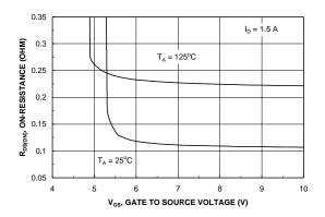
Figure 4. On-Resistance Variation with Gate-to-Source Voltage.
