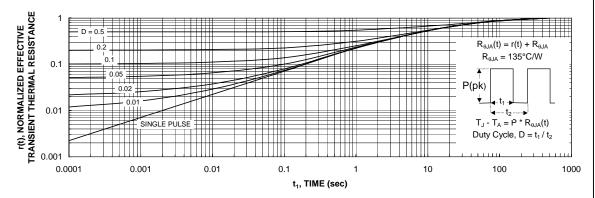
Figure 11. Transient Thermal Response Curve.
