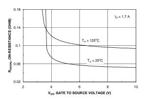
Figure 3. On-Resistance Variation with Temperature.
