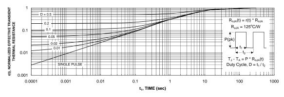
Figure 11. Transient Thermal Response Curve.
