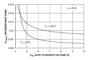
Figure 4. On-Resistance Variation with Gate-to-Source Voltage.
