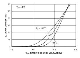
Figure 5. Transfer Characteristics.
