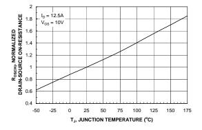
Figure 3. On-Resistance Variation withTemperature.
