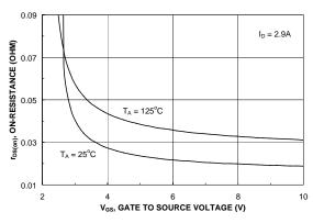
Figure 4. On-Resistance Variation with Gate-to-Source Voltage.
