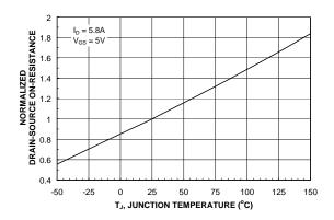
Figure 3. On-Resistance Variation with Temperature.
