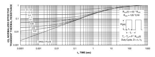
Figure 11. Transient Thermal Response Curve.
