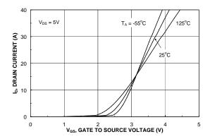
Figure 5. Transfer Characteristics.
