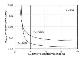
Figure 4. On-Resistance Variation with Gate-to-Source Voltage.
