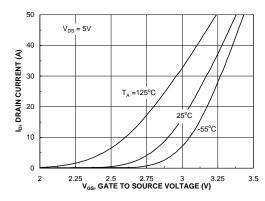
Figure 5. Transfer Characteristics.
