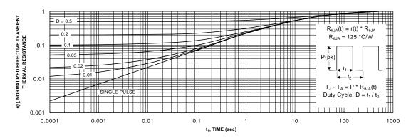
Figure 11. Transient Thermal Response Curve.
