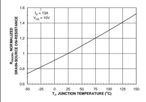
Figure 3. On-Resistance Variation with Temperature.
