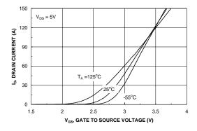
Figure 5. Transfer Characteristics.
