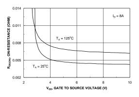
Figure 4. On-Resistance Variation with Gate-to-Source Voltage.
