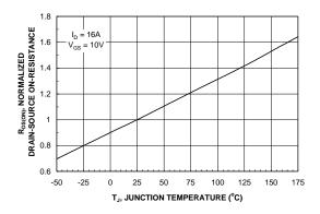
Figure 3. On-Resistance Variation with Temperature.
