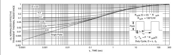
Figure 11. Transient Thermal Response Curve.
