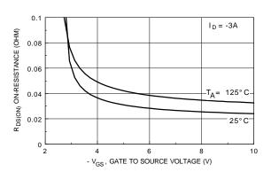
Figure 3. On-Resistance Variation with Temperature.
