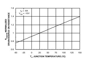
Figure 3. On-Resistance Variation with Temperature.
