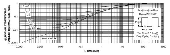
Figure 11. Transient Thermal Response Curve.
