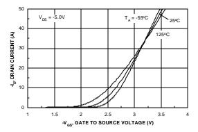
Figure 5. Transfer Characteristics.
