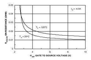
Figure 4. On-Resistance Variation with Gate-to-Source Voltage.
