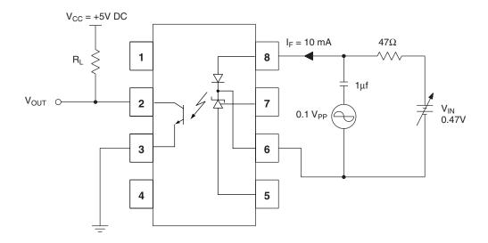
Fig. 7 Frequency Response Test Circuit
