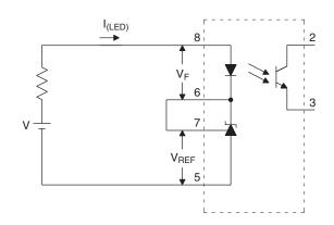
FIG. 1.  $V_{REF}$ ,  $V_{F}$ ,  $I_{LED}$  (min) TEST CIRCUIT
