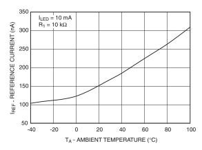
Fig. 12 Off Current vs Ambient Temperature
