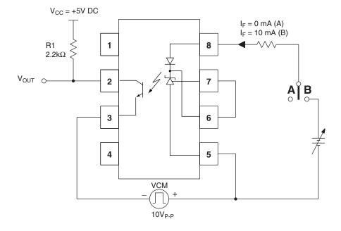
Fig. 8 CMH and CML Test Circuit
