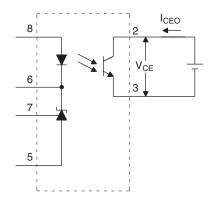
FIG. 5. I<sub>CEO</sub> TEST CIRCUIT
