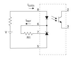
FIG. 3. I<sub>REF</sub> TEST CIRCUIT
