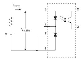
FIG. 4. I<sub>(OFF)</sub> TEST CIRCUIT
