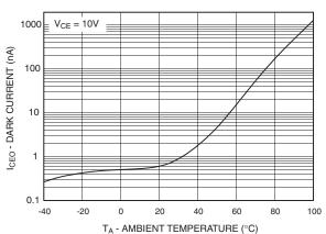
Fig. 15 Collector Current vs Ambient Temperature
