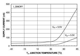
Figure 4. I<sub>SWITCH-OFF</sub> Current vs. Temperature
