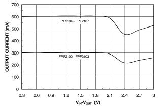
Figure 7. Current Limit vs. Output Voltage
