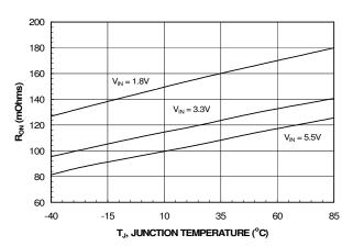
Figure 10.  $R_{(ON)}$  vs. Temperature
