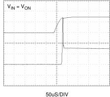
Figure 20. Current Limit Response (Switch power up to hard short)
