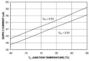
Figure 5.  $I_{LATCHOFF}$  vs. Temperature
