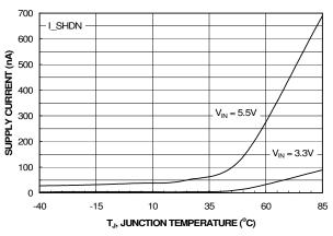
Figure 3. I<sub>SHUTDOWN</sub> Current vs. Temperature
