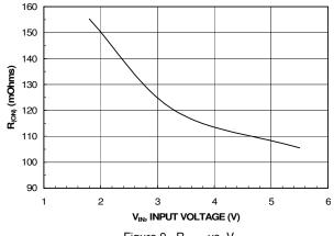
Figure 9.  $R_{(ON)}$  vs.  $V_{IN}$
