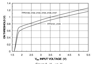
Figure 6.  $V_{IH}$  vs.  $V_{IN}$
