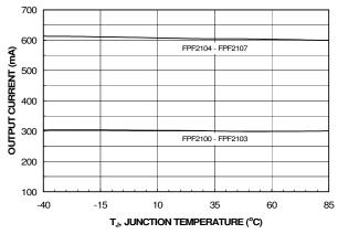
Figure 8. Current Limit vs. Temperature
