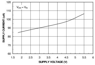
Figure 1. Quiescent Current vs. Input Voltage
