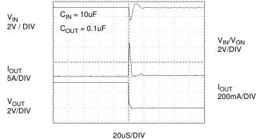
Figure 19. Short Circuit Response Time (Output Shorted to GND)
