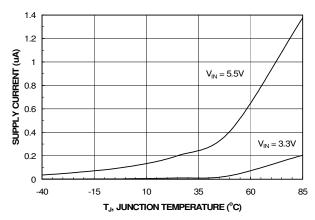
Figure 6. Reverse Current vs. Temperature
