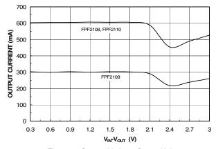
Figure 7. Current Limit vs. Output Voltage
