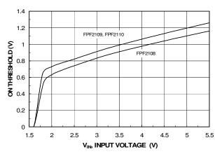
Figure 10.  $V_{IH}$  vs.  $V_{IN}$
