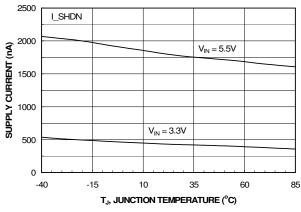
Figure 3. I<sub>SHUTDOWN</sub> Current vs. Temperature
