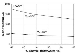
Figure 4. I<sub>SWITCH-OFF</sub> Current vs. Temperature
