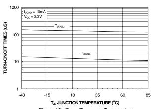
Figure 12.  $T_{RISE}/T_{FALL}$  vs. Temperature
