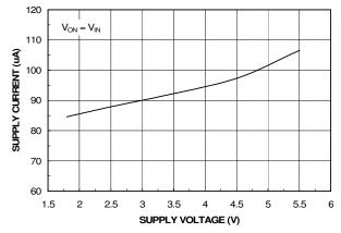
Figure 1. Quiescent Current vs. Input Voltage
