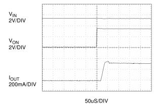
Figure 19. Current Limit Response Time (Output Shorted to GND by  $10\Omega$ , moderate short)
