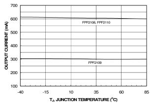
Figure 8. Current Limit vs. Temperature
