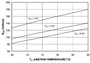
Figure 9.  $R_{(ON)}$  vs. Temperature
