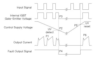
P1 : Normal operation - IGBT ON and conducting current P2 : Under voltage detection
