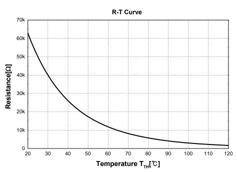
Fig. 5. R-T Curve of The Built-in Thermistor
