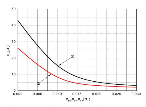
Fig. 6. R<sub>SC</sub> Variation by change of Shunt Resistors ( R<sub>SU</sub>, R<sub>SV</sub>, R<sub>SW</sub>) for Short-Circuit Protection
