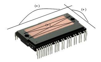
Fig. 7. Flatness Measurement Position of The DBC Substrate
