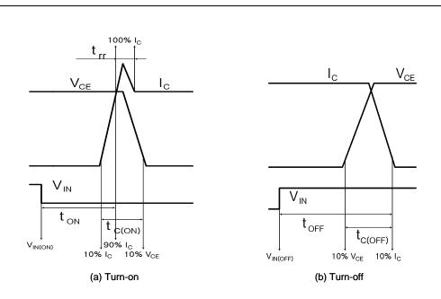
Fig. 4. Switching Time Definition
