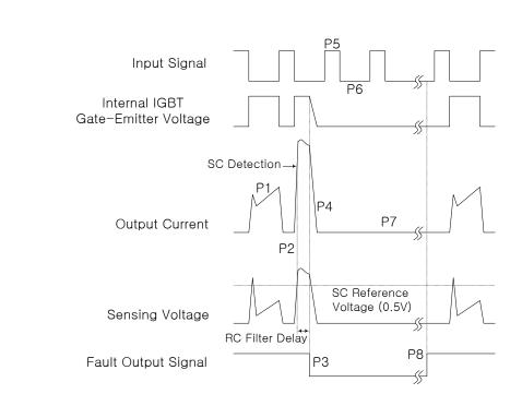
P1: Normal operation - IGBT ON and conducting currents
