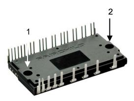
Fig. 8. Mounting Screws Torque Order (1  $\rightarrow$  2)
