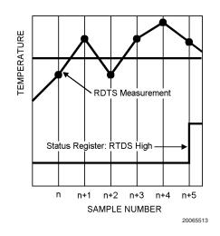
FIGURE 10. Fault Queue Temperature Response Diagram
