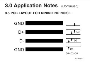
FIGURE 11. Ideal Diode Trace Layout
