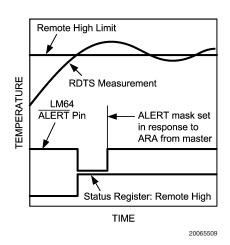
FIGURE 6. ALERT Output as an SMBus ALERT Temperature Response Diagram
