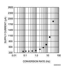
FIGURE 3. Supply Current vs Conversion Rate
