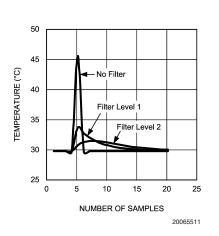
FIGURE 8. Impulse Response of the Digital Filter
