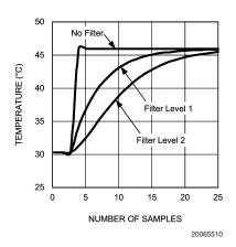
FIGURE 7. Step Response of the Digital Filter
