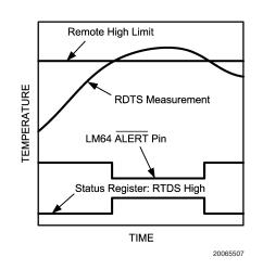
FIGURE 4. ALERT Output as Temperature Comparator Response Diagram
