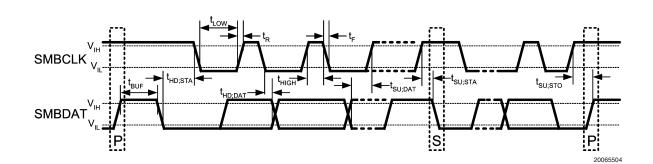
FIGURE 1. SMBus Timing Diagram for SMBCLK and SMBDAT Signals
