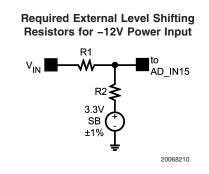
The +3.3V standby voltage is used as a reference for the level shifting. Therefore, the tolerance of this voltage directly effects the accuracy of the -12V reading. To minimize ratio errors, a tolerance of better than  $\pm 1\%$  should be used. It is recommended that the equivalent thevenin resistance of the divider is between 1k and 7k to minimize errors caused by leakage currents at extreme temperatures. To calculate the ratio of R1 to R2 use this equation:
