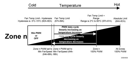
FIGURE 1. Fan Activity above Fan Temp Limit
