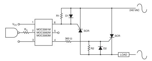
Figure 12. Inverse-Parallel SCR Driver Circuit
