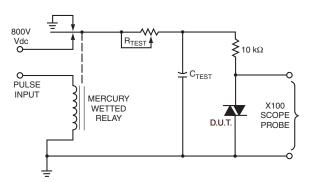
Figure 9. Static dv/dt Test Circuit
