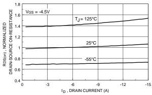
Figure 3. On-Resistance Variation with Temperature.
