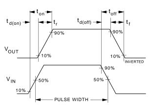
Figure 12. Switching Waveforms.
