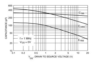
Figure 9. Capacitance Characteristics.
