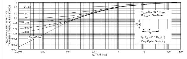
Figure 17. Transient Thermal Response Curve.
