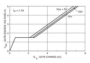
Figure 10. Gate Charge Characteristics.
