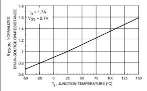
Figure 3. On-Resistance Variation with Temperature.
