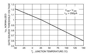
Figure 6. Gate Threshold Variation with Temperature.
