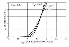
Figure 5. Transfer Characteristics.
