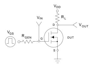
Figure 11. Switching Test Circuit.
