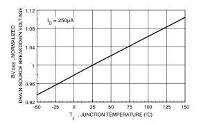
Figure 7. Breakdown Voltage Variation with Temperature.
