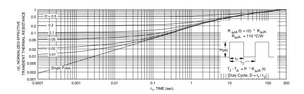
Figure 11. Transient Thermal Response Curve.
