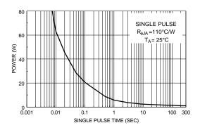
Figure 10. Single Pulse Maximum Power Dissipation.
