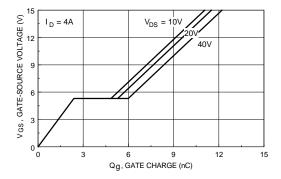
Figure 7. Gate Charge Characteristics.
