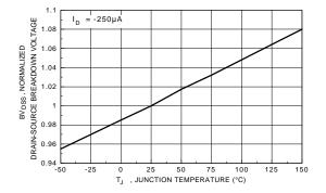
Figure 7. Breakdown Voltage Variation with Temperature.
