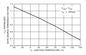
Figure 6. Gate Threshold Variation with Temperature.
