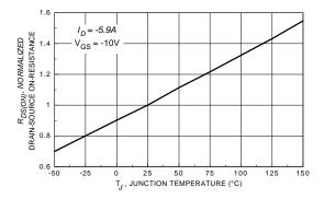
Figure 3. On-Resistance Variation with Temperature.
