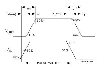
Figure 12. Switching Waveforms.
