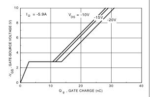
Figure 10. Gate Charge Characteristics.
