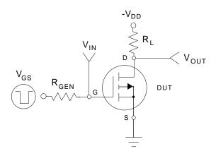
Figure 11. Switching Test Circuit.
