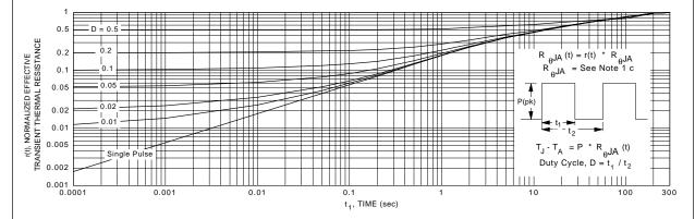
Figure 15. Transient Thermal Response Curve.
