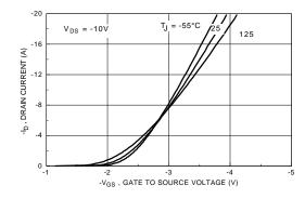
Figure 5. Transfer Characteristics.
