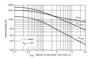
Figure 9. Capacitance Characteristics.
