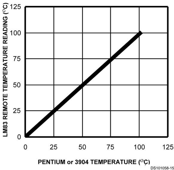
**Pentium or 3904 Temperature vs LM83 Temperature Reading**
