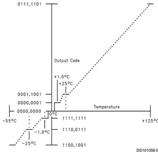
FIGURE 2. Temperature-to-Digital Transfer Function (Non-linear scale for clarity)
