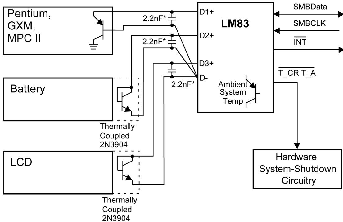
\*Note: 2.2nF Capacitors must be placed as close as possible to D+ and D- pins of the LM83.
