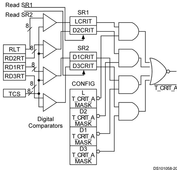
**FIGURE 7.  $\overline{T\_CRIT\_A}$  output related circuitry logic diagram**
