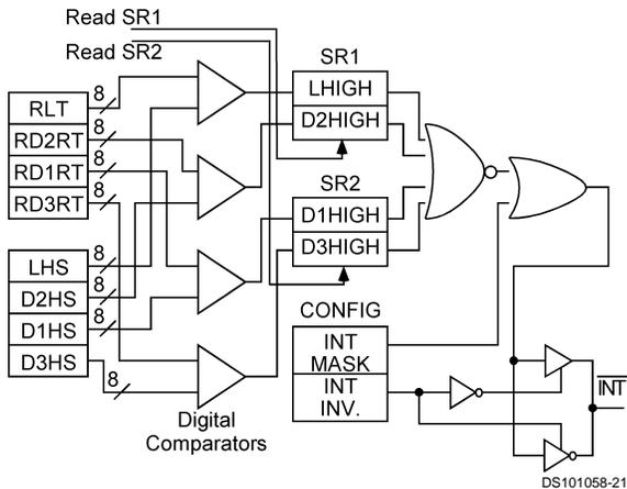
**FIGURE 5.  $\overline{INT}$  output related circuitry logic diagram**
