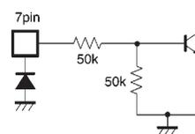
$t_m \leq 125 \mu s$  \*3 Equivalent circuit diagram for mute pin
