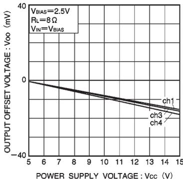
Fig.10 Power supply voltage vs. output offset voltage
